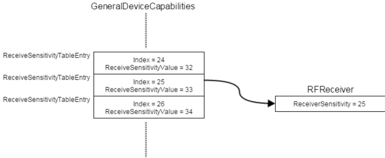
Conversely, given the `ReceiverSensitivity` field from the `RFReceiver` parameter, the effective receive sensitivity level in dBm can be determined as follows:
