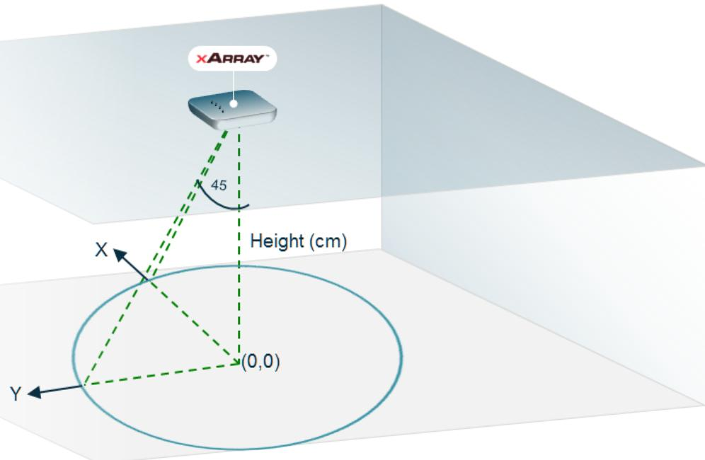
The following figure shows an example of how Location and Orientation would be specified for an example configuration.
