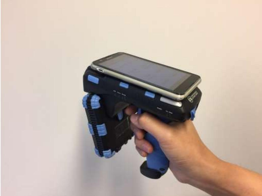
CS108-2 can also be controlled via the USB connection by a PC. In this case, the Bluetooth connection is not used. The control commands enter via the USB cable. The application is on a PC.
