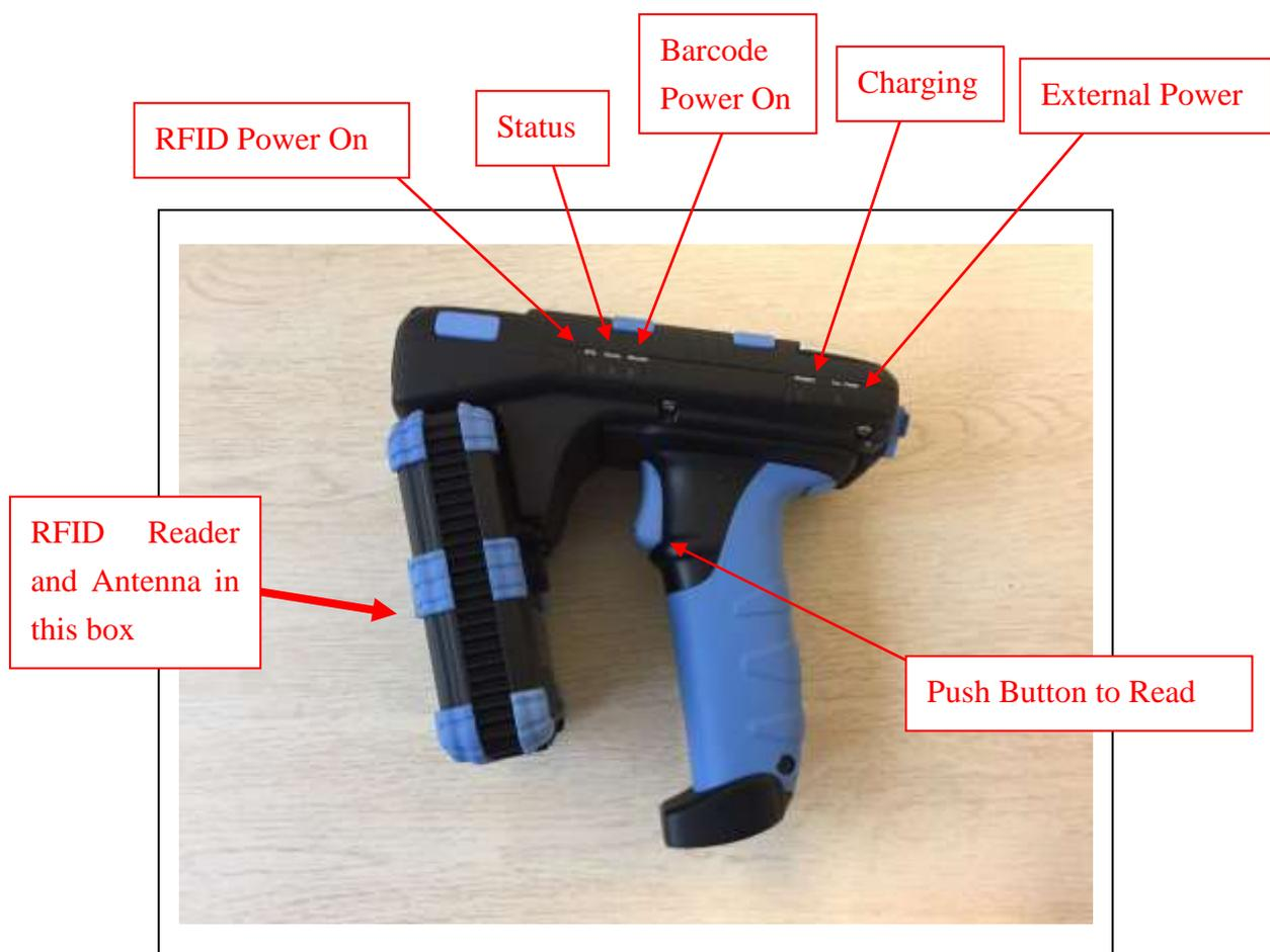
**Figure 4-2 CS108-2 Reader Left Side View**
