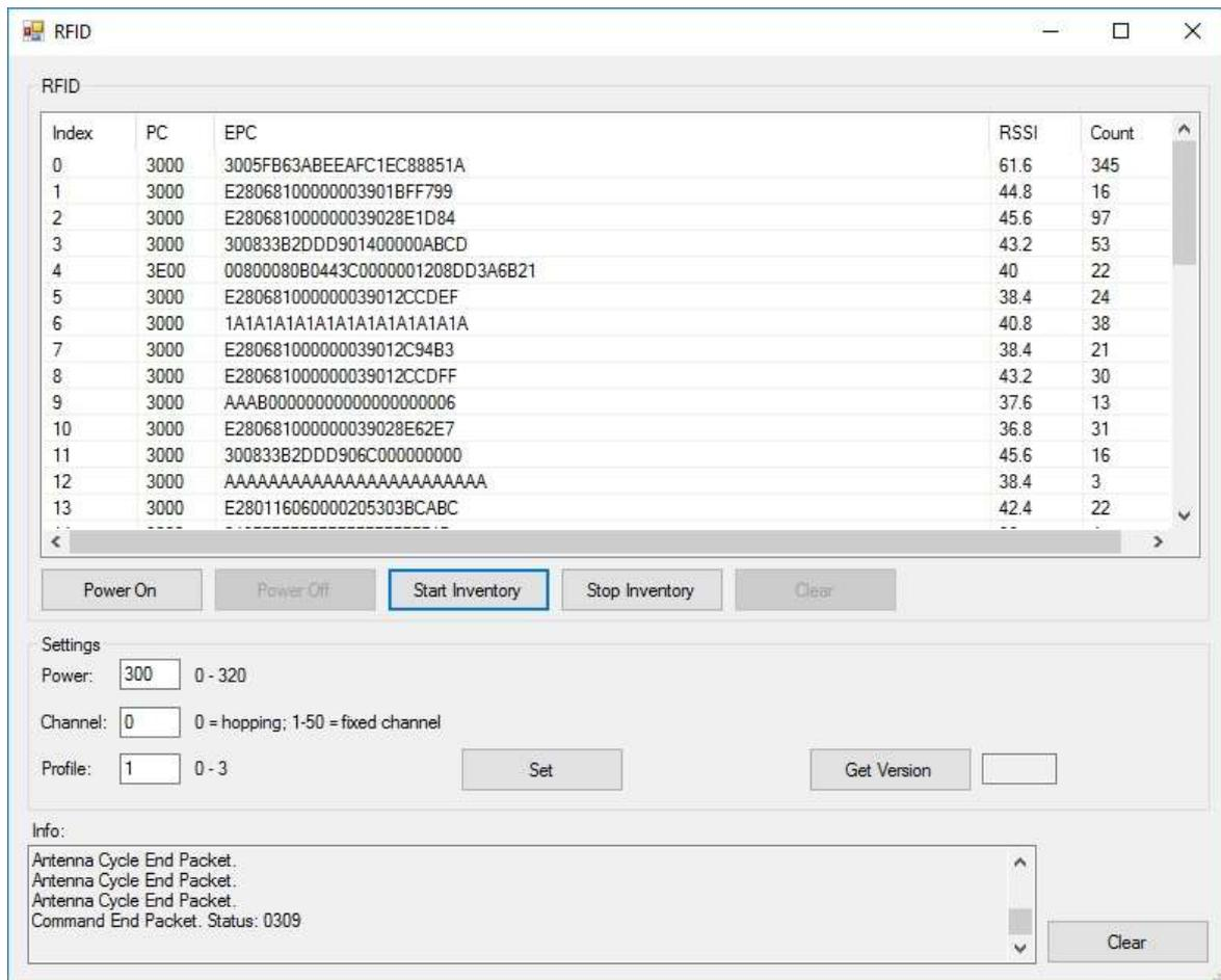
Figure 4-5 PC Application Screen – controlling CS108-2 via USB
