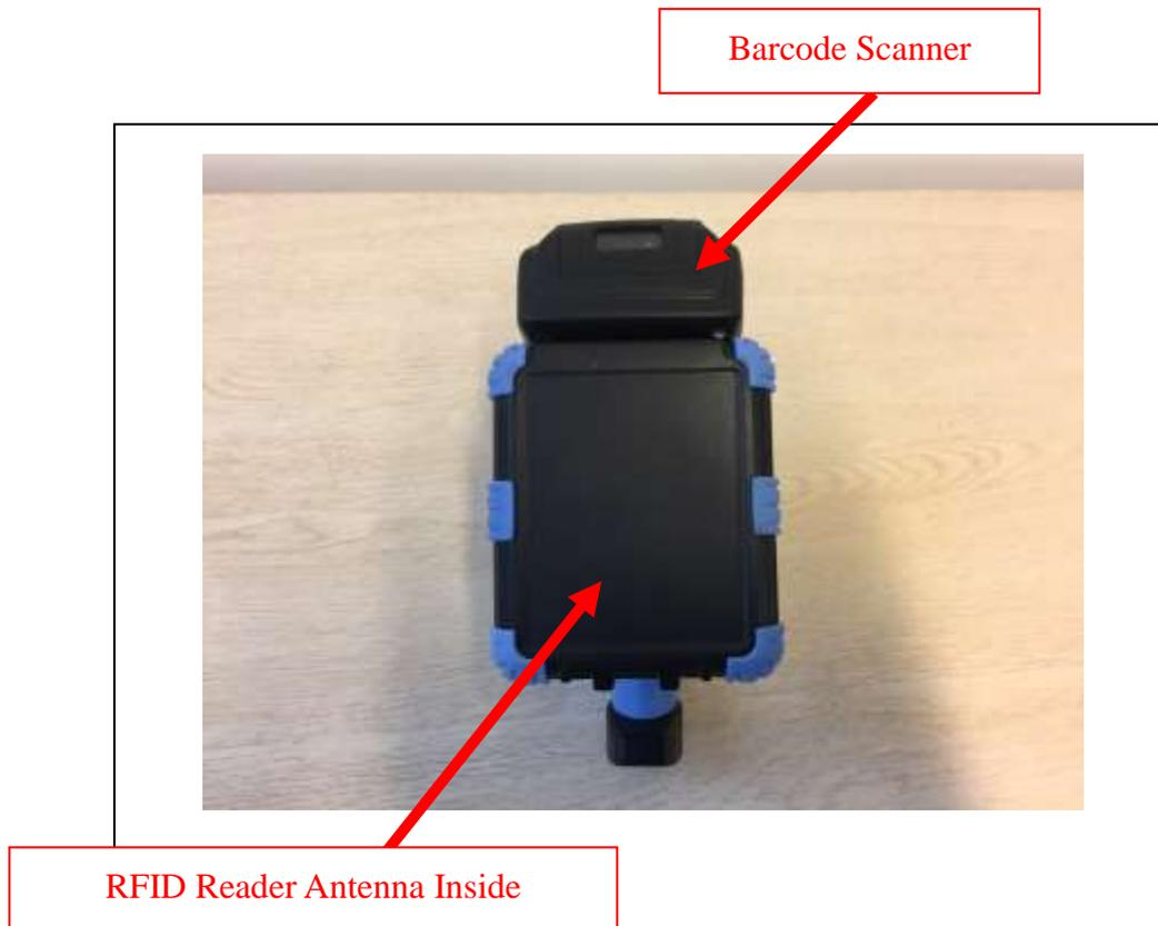
Figure 4-1 CS108-2 Reader Front View
