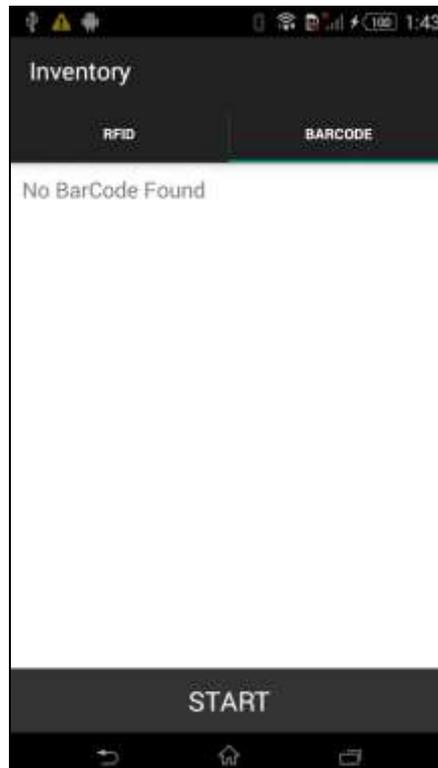
Press the **START** button. At this point, the red LED of the barcode reader should lit up to help you aim your CS108 barcode reader onto the barcode. A focused circular dot should appear. That is where the distance of the barcode should be with respect to the reader.
